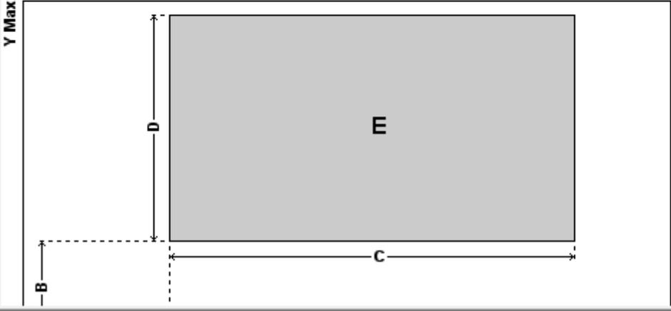
The diagram shows a coordinate system with 'Y Max' on the vertical axis. A dashed line indicates the origin 'B' at the bottom-left corner. A horizontal dimension 'C' is shown from the origin to the right edge of the printing area. A vertical dimension 'D' is shown from the origin to the top edge. A shaded rectangular area 'E' represents the printing area, starting at the origin and extending to dimensions C and D.
