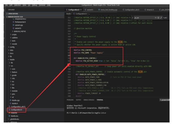
2. Take SKR-PRO-V1.1 as an example, open the pins\_BIGTREE\_SKR\_PRO\_V1.1.H file in the order shown in the figure, then find "#define PS\_ON\_PIN PF13" in the file and remove the previous mask "//". PF13 is the shutdown signal pin, which can be changed according to your own needs, as shown in the figure:
